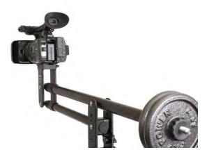
If you keep your hands on the jib, you may be able to operate it without the tilt or pan brakes tightened. If you need to take your hands off the jib, you may want to tighten the tilt and/or pan brakes to hold position. These brakes are not hard-stop mechanisms, they are soft-stops that can be pushed-through.
